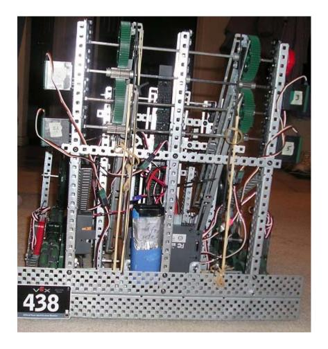
We needed a better solution. PID control was popular, but we didn't understand the calculus, so we searched for pre-written code on the Vex forum under the "code" tab. Using a downloaded program, the arm twitched and moved without driver input. The documentation said to "tweak" the gain values for the P, I, and D components, but we couldn't make it work by trial and error, so we looked for a simpler solution, one we could understand.
