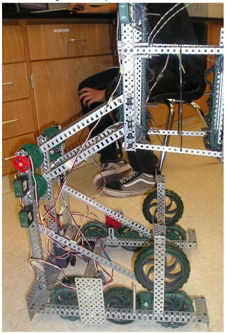
We wanted the arm to stay up without input, rather than forcing the driver to continually push the "up" button. Our mentor showed us how to search for solutions on vexforum.com (create an account, then use the "search" tab) and found a thread called "Having a motor HOLD its position."
