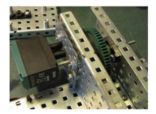
This concept can be seen on our robot. You can see that the wheels and transmission is assembled and that the motors are attached to a chassis. In the event of a motor failure we only need to remove these three screws, remove the tie wraps holding the cables and the motors can be easily removed. All the remaining assembly, gears, axis and wheels remain untouched. Reverse the steps with your spare chassis and you will be back in the competition in no time.
