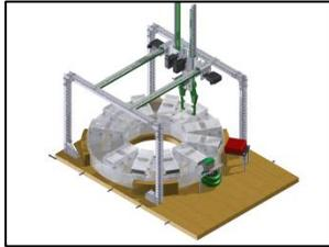
them into the mobile robot's socket. A barcode scanner is used to find the proper seed module. The barcode provides planting and watering information for that seed type. A section of the monorail track inside the seed module changer rotates to allow the robot to swing its arm into the proper position for seed loading. This also allows the robot to move its arm from one side of the track to the other.
