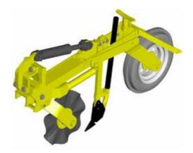
The Coulter takes the seeds from a hopper and plants them in the ground. The Leading Disc cuts a thin slot in the ground. The Tine in the centre delivers the seed at the correct depth. The entire frame has a hydraulically adjustable ground pressure spring on the top to force the rear tyre to follow the contour of the ground. The final hydraulic ram at the front allows the entire unit to be raised for road travel.
