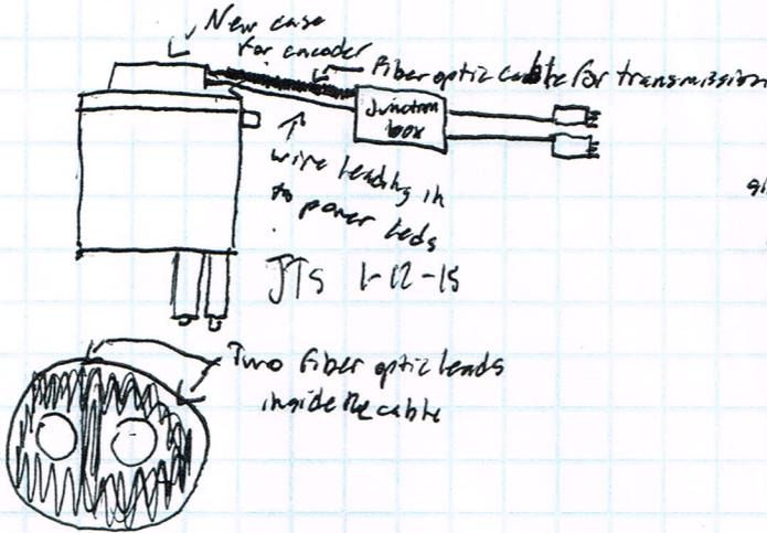
After the fiber optic leads reach a junction box several inches down the cable, they are converted into electronic signals using photoresistors. After the photoresistors, a ~~low~~ simple low pass filter using a capacitor filters all high frequency noise off the signal, and a toroid on the cable filters even more noise, resulting in a clear signal ready for the cortex to read.
