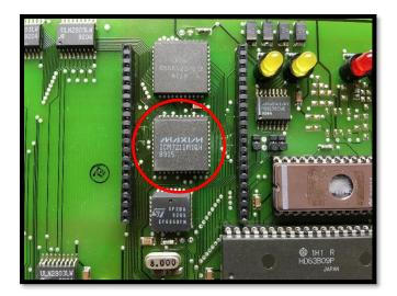
ICM7211MIQH converts Binary Coded Decimal to 7 segment digits on the 4-digit LCD temperature display.
