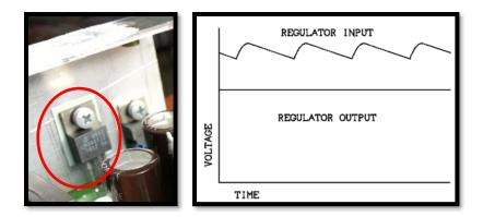
An LM340T12 voltage regulator produces a constant 12Vdc output. Unwanted energy is dissipated as heat through an aluminium heatsink.
