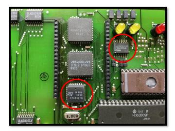
An EF6850FN and MAX232CWE provide a serial port for temperature history download.
