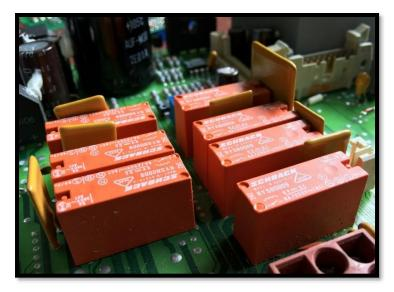
Electromagnetic relays switch high power refrigeration plant circuits controlling fans and the compressor.
