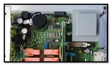
The AC to DC power supply is made up of a bridge rectifier, smoothing capacitor and linear voltage regulator.
