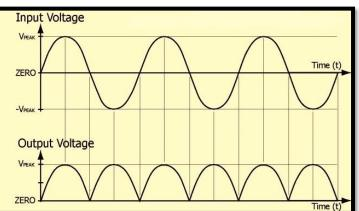
The KBU4B bridge rectifier converts AC to DC using 4 diodes.
