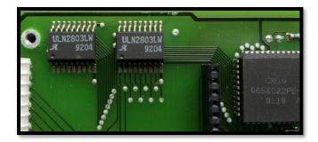
I/O interfacing IC G65SC22PE connected to ULN2803 drivers control relays and LEDs.
