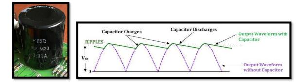
The 10000uF capacitor smooths the bridge rectifier output.
