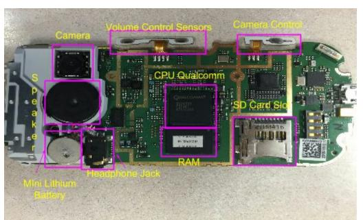
brightness. Last but not least is the LG battery which is the main power source.
