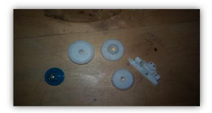
The gears and the rack gears are responsible for transferring the movement from the motors to move the cd housing inside and outside the CD rom.
