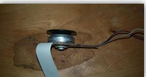
The motor and the magnet are responsible for rotating the CD with a high speed to make the laser circuit read it.
