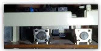
They are used for giving the commands to the motors to make the CD housing move inside and outside the cd rom and they are used to navigate between audio files in the CD.
