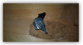
This unit is responsible for reading the CD and sending the data to the processing board.
