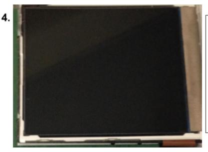
This display is an Ilitek 19335: Single-chip 320\*240 pixel display driver (2.8" diagonal)and displays a resolution of 140 dots per inch (DPI); 16-bit color. This supplier: llitek makes displays used in Apple products and Windows computers (see link in Sources)
