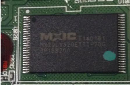
Since the 1980s, Flash ICs such as this Macronix integrated circuit (shown above) have been a vitally important integrated circuit in consumer electronics. These ICs come with millions of tiny transistors on a silicon chip a few millimeters square. This Flash IC has a 32 Mbit capacity that can be segmented into various sizes. They save data permanently unlike other types of memory ICs, which retain data only as long as the power stays on.
