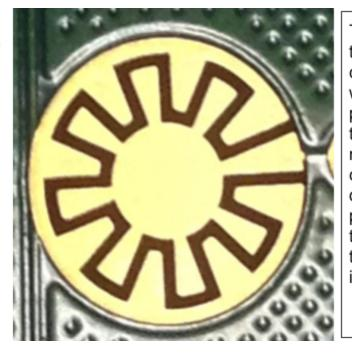
This is a close up look at one of the 50 touch sensors on the calculator. The touch senses whether the button is being pushed or not in binary data. It then transfers this data to the microprocessor, which computes an equation from the data of which buttons are pressed. The microprocessor then sends the final answer to the llitek display, which displays it.
