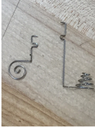
Metal Wires that connect batteries to circuit
