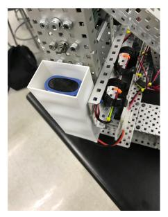
conducted to ensure that the part was securely fastened onto the robot and did not fall off. Our testing resulted in success as the case kept the battery protected, and we were able to plug the cable in through the hole in the case and into the cortex with relative ease. Though it is not feasible to test the ability of the case to remain secure while being hit by another robot's scoop in the robotics classroom, we are confident in its abilities to remain attached during that
