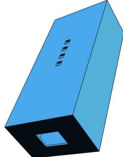
screwed and nylocked onto the robot would be the solution to our problems. This case fully envelops the battery, and is firmly secured onto the robot itself, preventing the scoop of another robot from knocking the battery off and potentially damaging it. In order to create this case, we extensively measured the VEX robotics batteries so that we could create a design that fit the battery securely. In addition to measuring the battery itself, we also
