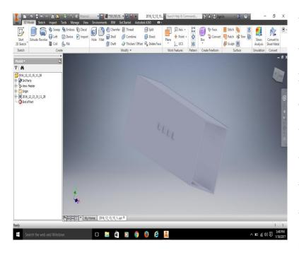
we then used them to make a hole on the bottom of the case for the plug to come out. We also had to create screw holes in the back of the case to mount the case onto the robot. Taking into account the weight of the battery and that of the case, we decided that four screw holes would be more than
