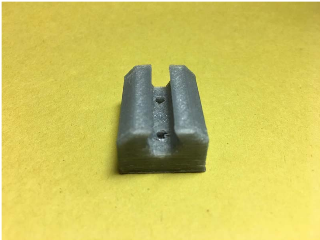
8. Front-top view of the 3D printed standoff slide truck
