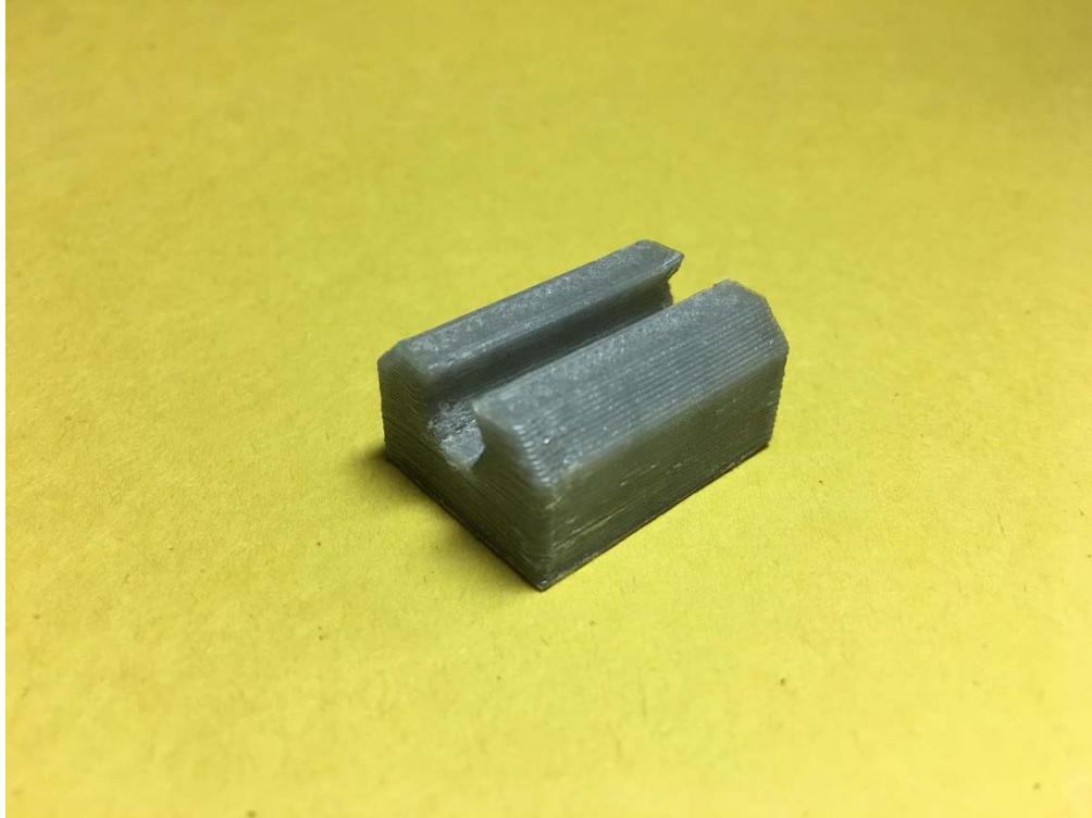
7. Isometric view of the 3D printed standoff slide truck
