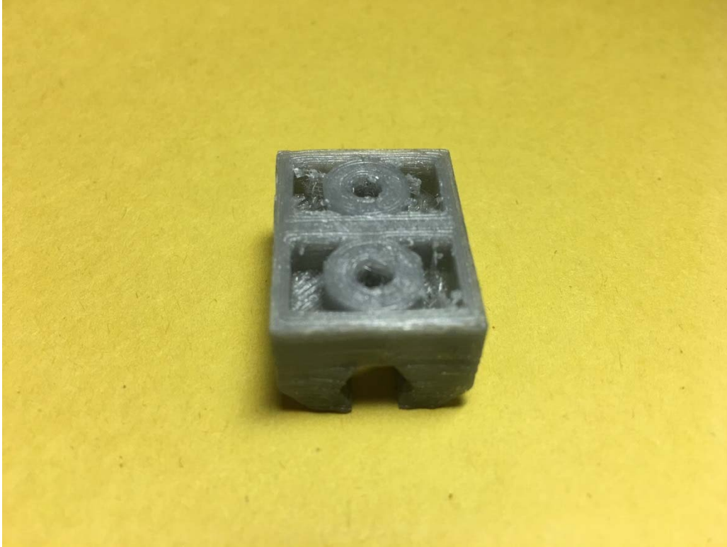
9. Bottom view of the 3D printed standoff slide truck
