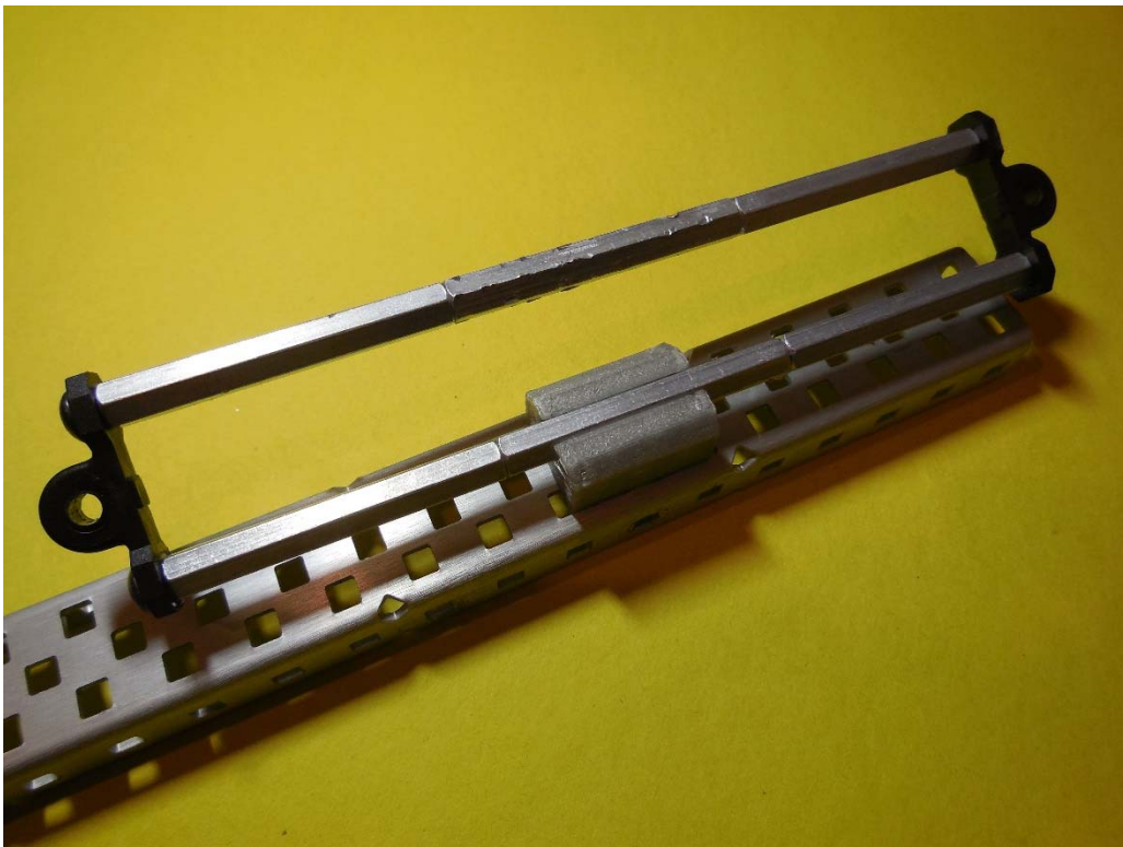
10. An angled sliding mechanism using the standoff slide truck
