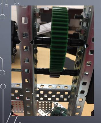
The gear that moves the arm up and down
