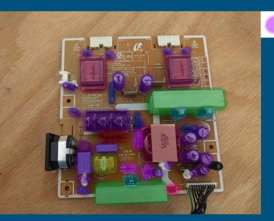
Diodes used to keep current flowing in the direction it's supposed to
