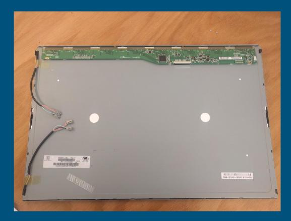
We inferred that they are driving circuits for the LCD as we could not find any datasheets on most of the IC's
