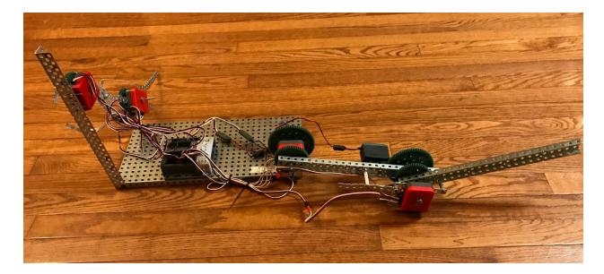
The encoders on the sleeve record these movements as a measure of degrees, and then the encoders on the robotic arm read the position of the arm and determine whether the specific joint they were on was less or above the sleeve encoders value. The cortex then sends a signal for the motors to turn, depending on the encoders value.
