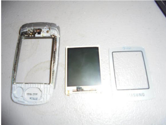
The UV Screen, Face, and Frame
