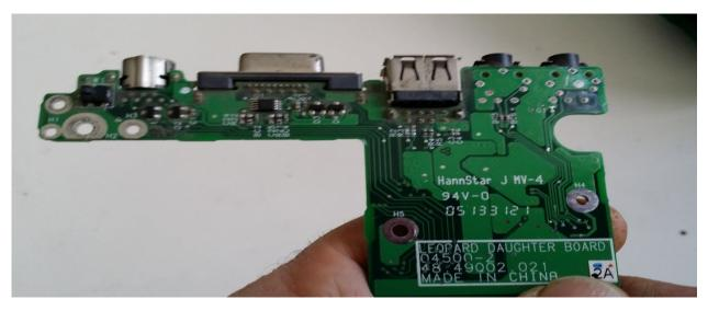
A daughterboard is an extension of a motherboard & have plugs, sockets, pins, connectors, or other attachments for other boards.
