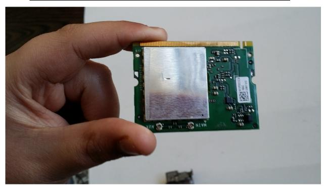
2. Integrated wireless Chip for Mini PCI IEEE 802.11b/g WLAN device-Wireless LAN card
