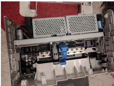
Figure 11: The back panel was removed to gain access to internal components and determine most efficient and safe method to remove the printed circuit boards.
