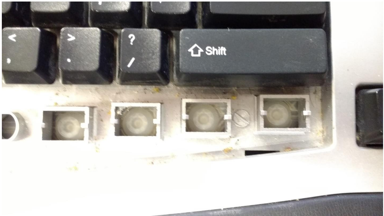
Some keyboard keys removed. The rubber dome buttons are visible here.
