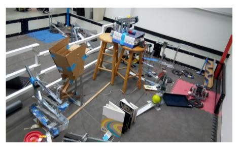
board to come up with a better idea. Eventually, however, we succeeded. Our Rube Goldberg consisted of a ping pong ball that was carried down a conveyor belt and placed into a launcher, which sent it into a funnel. The ball ran down a switchback leading from the funnel to a light sensor that triggered a
