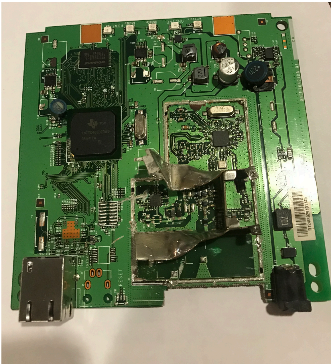
Final disassembly of SURFboard SB6121, a Motorola modem, with TI transceiver number TNETC4830ZDWG
