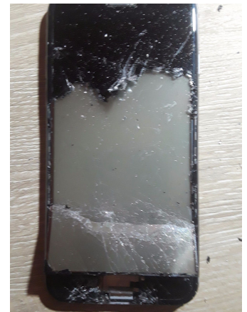
This is a glass rectangle that was under the screen. It senses the heat and pressure from your hand.
