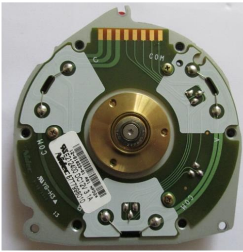
Thin, small motor used to turn the take-up reel
