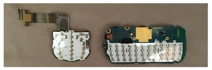
The main circuit board (right) had 48 buttons for letters, numbers etc. On the other circuit board (left) there were 23 buttons.
