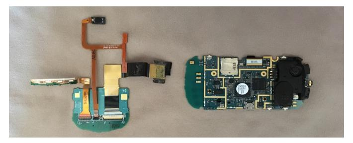
On the other side of the circuitboard we found (right) a micro SD card reader, a micro USB in port, we are pretty sure we found some storage banks, and we also found four small buttons (volume, sleep, home). We also found the inverter. On the other circuit board (left) we found the wire that connected the two boards and that runs the power through the whole phone. This was also where the output wire of the speaker and the volume buttons were as well as the output wire
