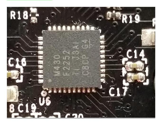
Texas Instrument "MSP430 microcontroller" reads the users inputs and transmits them wirelessly or through the tether port. The microcontroller uses ultra-low-power. The architecture, combined with five low-power modes is optimized to achieve extended battery life in portable measurement applications.
