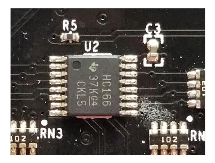
On further research we found another Texas Instrument an "8-Bit Parallel Load Shift Register HC166" which shifts data to serial output. Parallel-in access to each stage is provided by eight individual direct data inputs that are enabled by low level shift/load input. It is fabricated with silicon gate CMOS technology. It consumes low power with standard CMOS IC, and can operate at speeds comparable to the equivalent low power Schottky device.
