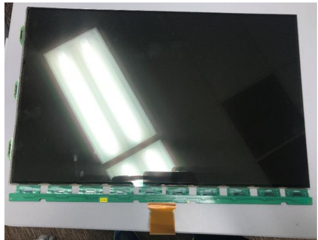
(left) This board was connected to the main LCD panel via a ribbon cable
