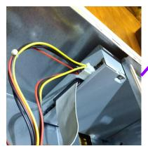
Optical Disc Drive: is a disk drive that uses laser light or electromagnetic waves within or near the visible light spectrum as part of the process of reading or writing data to or from optical discs.
