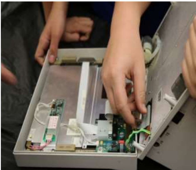
Figure 7: (At Left) Manjot is detaching a ribbon cable that held the front housing assembly to the rear housing assembly.
