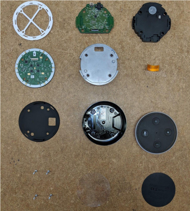
This is all of the parts that make up the Echo Dot.
