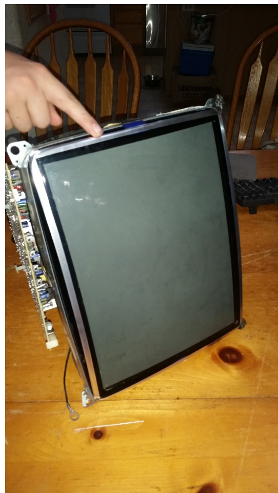
Front of monitor with shell removed
