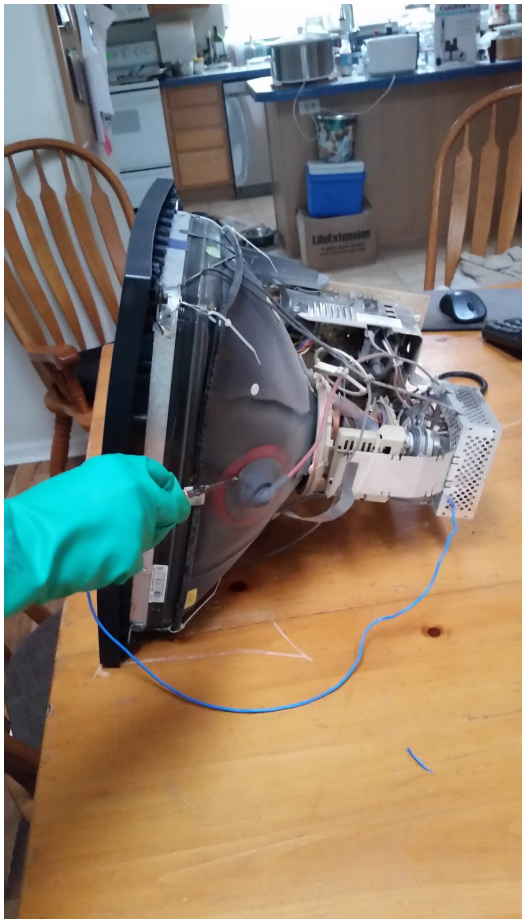
Discharging 2 (for safety) - different screwdriver/ground
