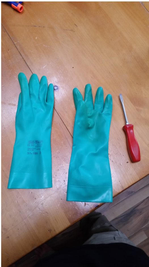
Rubber gloves and screwdriver used for safety and discharging
