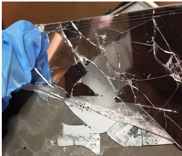
Peeling the E-ink display off the midframe.
