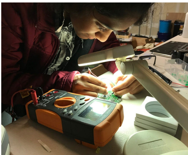
Roshni using a multimeter to identify components based on resistance.
