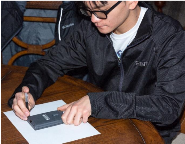
Figure 1: Removal of the battery cover and the four screws from the back cover of the device
