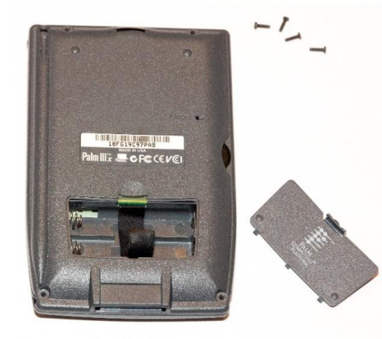
Figure 1: Removal of the battery cover and the four screws from the back cover of the device
