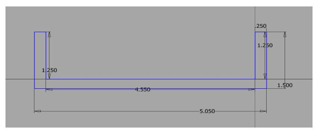
1. We made the outline of the license plate flipper to be just the right size to fit a license plate. And we extruded it .550 inches.
