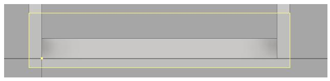
2. We needed a back wall to make the license plate flipper more rigid and so the license plate would not fall out so we made a sketch outlining the frame and extruded it .10 inches
