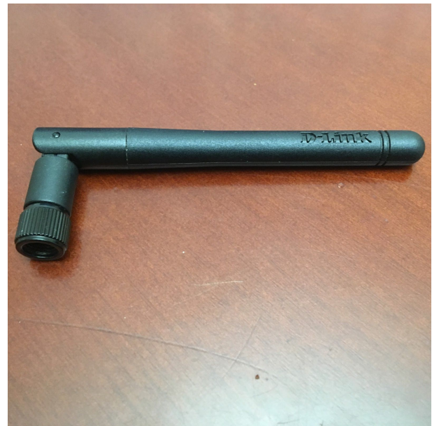
An Omnidirectional Antenna which amplifies signals in all directions in one plane, with the decreasing as you go down.
