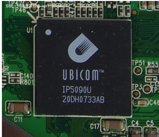
Ubicom IP5090U, revealed under the heatsink
