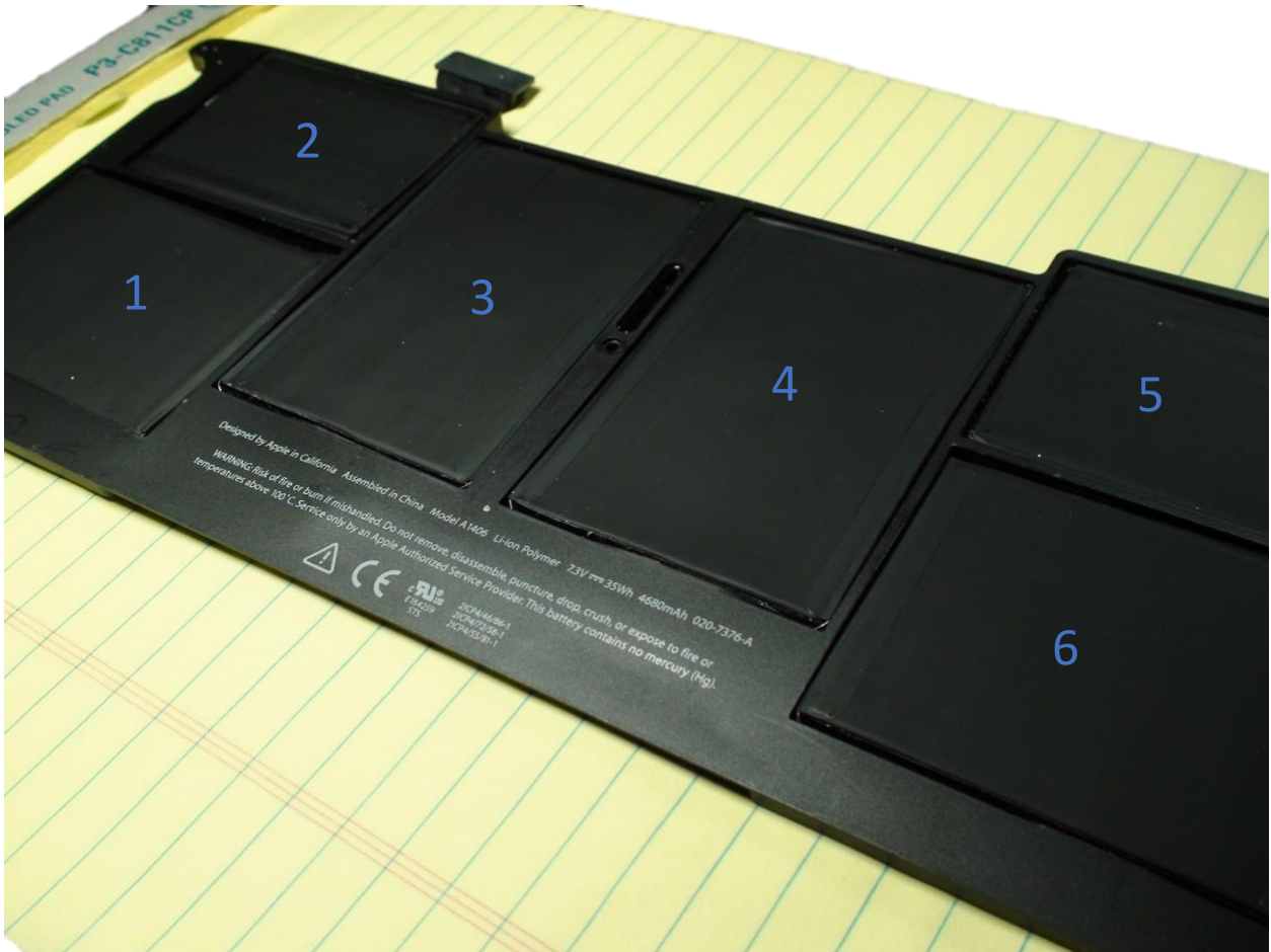
Figure 3 A 6-cell 4680mAh Battery
