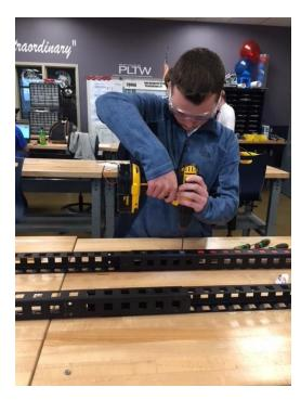
Noah drills through the hardened steel stand in order to push the securing bolt through. The steel was so sturdy it broke one of our drill bits!
