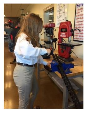
Lucy, midswing in an attempt to bend the bottom part of the metal to a 90 degree angle so we can properly secure it to the baseplate.
