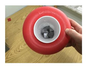
styrofoam cup and placed weights inside of it to simulate the weight of the damp soil and plant the device would hold. When testing we learned that the ring was capable of holding more than enough weight to be sufficient to carry a plant and soil. The test design can be seen in the picture above. In our final design we will be using a plastic cup to make sure the cup does not break and leak soil.
