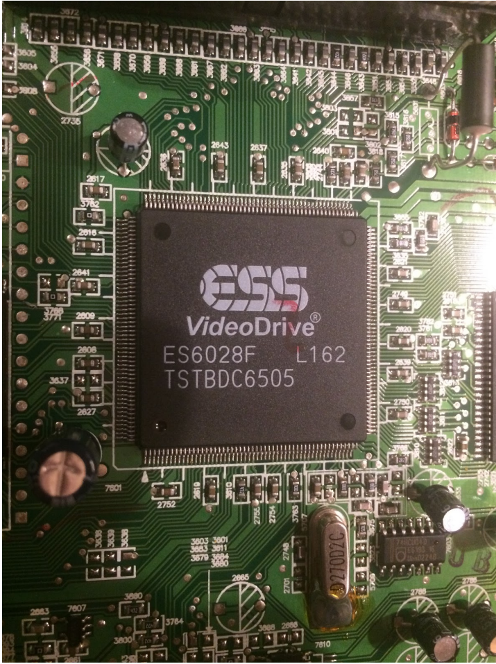
This is the ESS VideoDrive that is used for the display. It is located near the center of the board.
