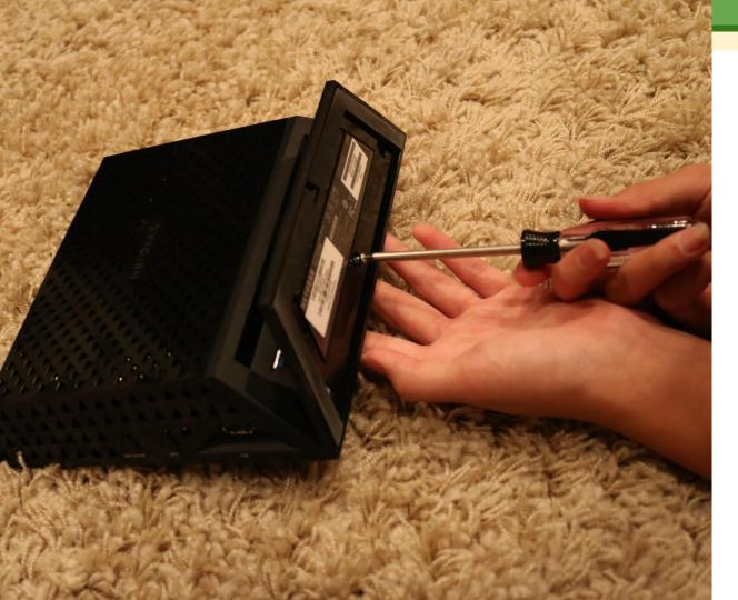
WE HAD TO USE A SPECIAL SCREWDRIVER CALLED A TORX SCREWDRIVER. IT HAS A 6-POINT STAR SHAPED PATTERN ON ITS HEAD.
