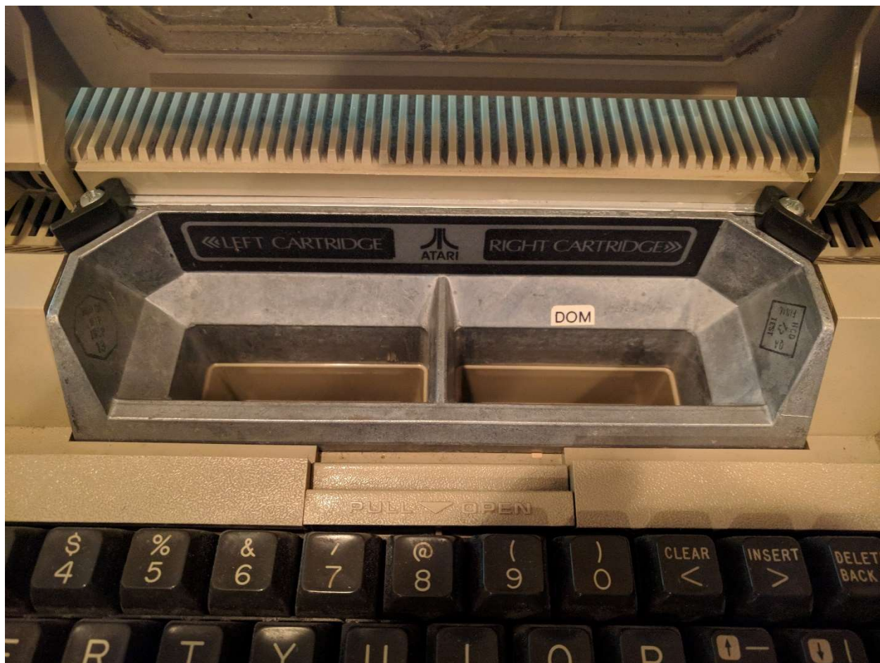
The Atari 800's bizarre double cartridge slots. The right slot was never really used for anything.
