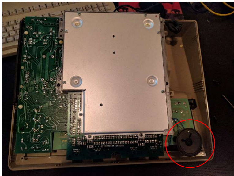
There's not much to see yet, except for an obnoxious speaker that clicks every time a button on the keyboard is pressed. It is circled in red.
