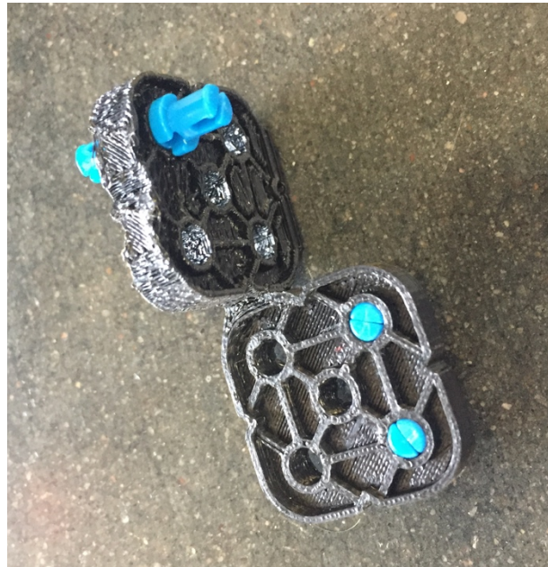
Photo 6 Printed 3D piece. We tested if the pins would fit and they did. Quality not perfect.
