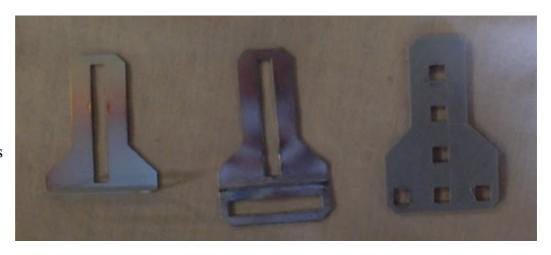
We used fusion 360 version 2.03800 to create our T-piece. Even though it is a simple design, we feel it would work well as a T-shape metal plate. There are already flat VEX pieces but this is a shape that is needed, as there are many angled gussets and corner gussets, but there are no T-shape ones, which is what we need.
