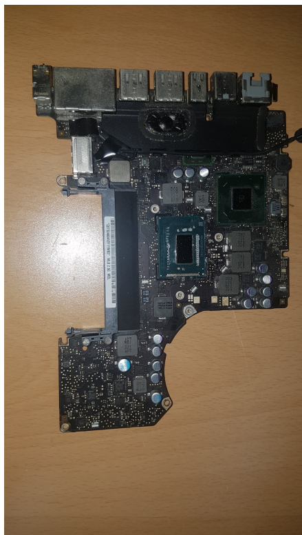
The Logic Board, Detached Cooler for the CPU and the Platform Hub.
