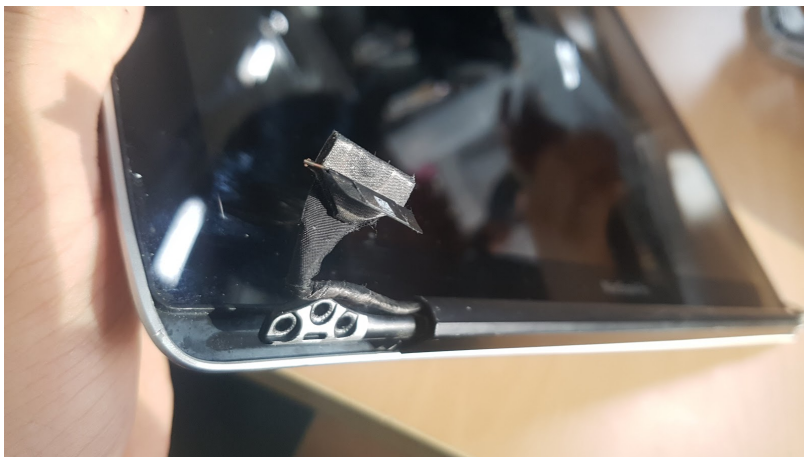
Detached LCD, providing display and GUI for the calculations done in the logic board for user integration.
