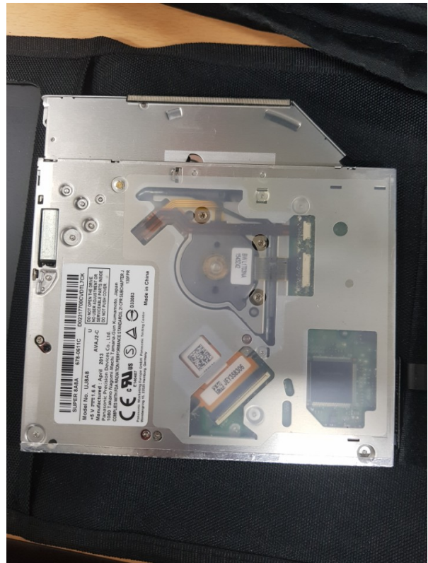
Removed Optical Drive, or ODD, allowing CD or DVD read/write ability for the MacBook pro.
