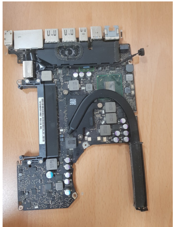
The Logic Board of the computer, without the cooler taken off. Responsible for the connection of all components in one specified spot.
