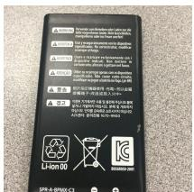
• The 3.7V 1300mAh 5Wh Li-Ion battery is what powers the 3DS XL on its battery life is 3 - 5 hours depending on the intensity of the game and how much power is needed from the CPU/Chip.
