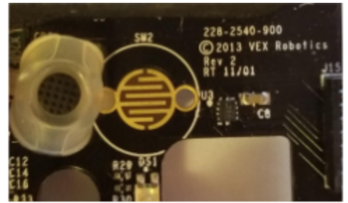
Figure 4: close-up of membrane switch
