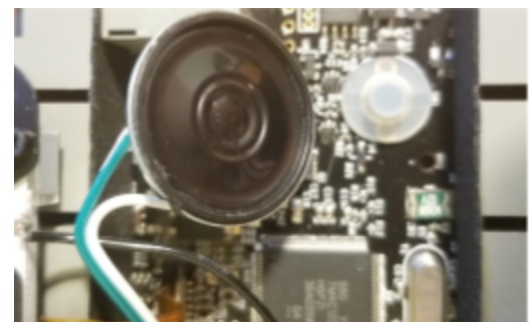
Figure 5: close-up of 5 watt speaker behind LCD housing
