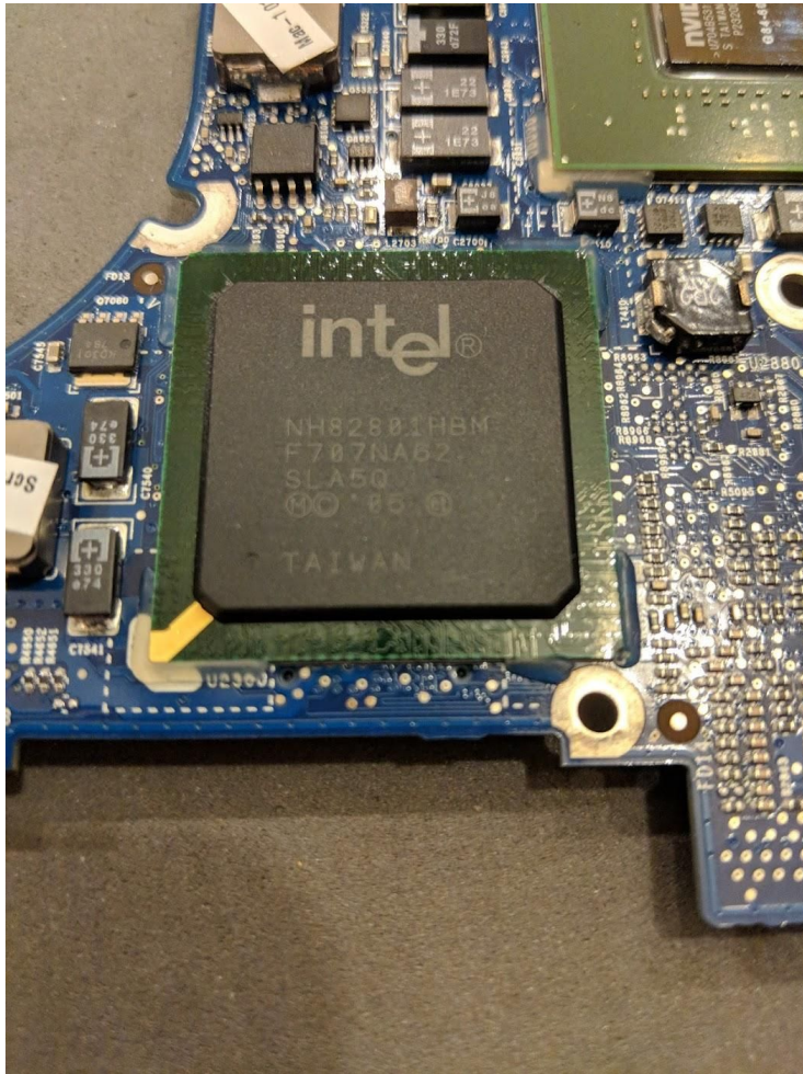
Intel NH82801HBM. This connects the PCI, BIOS, and the Super I/O to the North Bridge.
