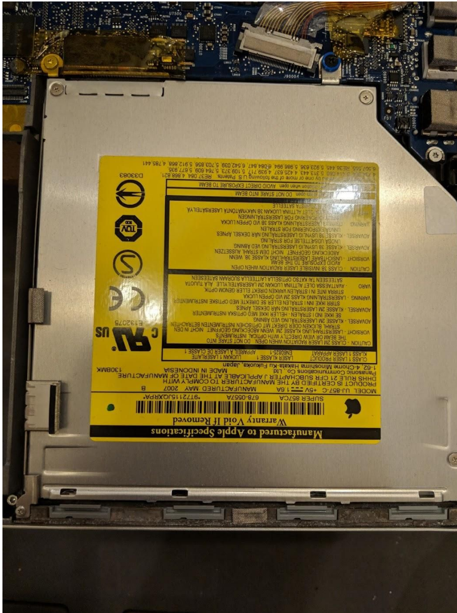
Panasonic Superdrive. This is a CD/DVD read-write drive. It is also capable of reading and writing CD's/DVD's, something today's laptops do not include.
