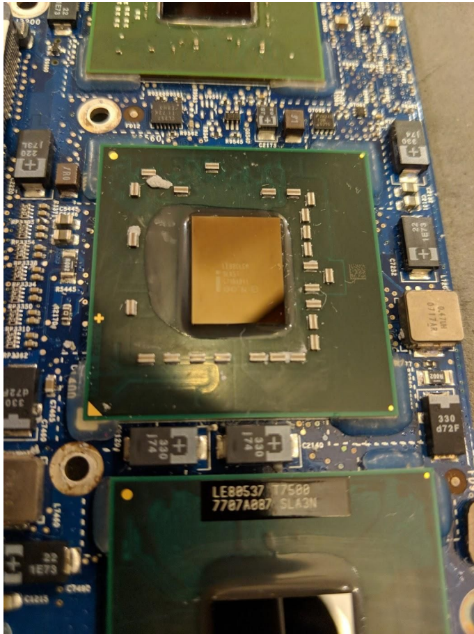
Intel LE88CLGM. Memory controller. This connects the CPU, South Bridge chip, memory, and graphics.
