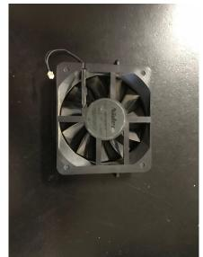
The fan cools down the system. It connects to the motherboard through the connector. The motherboard tells it to activate when the electronics overheat.
