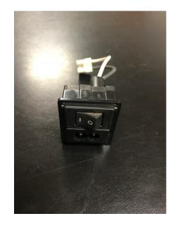
This device allows power to flow from the power source board to everything else. It connects to the power source board through the connector.
