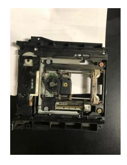
The picture above shows the optical disc drive. It reads the data off any discs inserted into it. It can play DvD's and PS2 games
