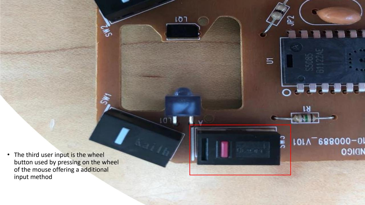
The motion of the scroll wheel is sensed by the optical encoding sensor similar to the Vex axle encoder
