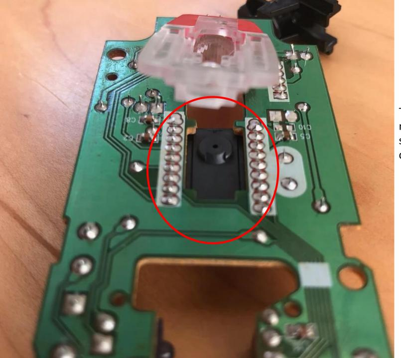
The infrared sensor interprets the movement of the magnified light on the surface sending the information to the computer.
