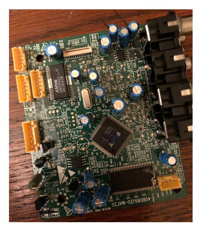
we believe this major pcb is the main unit for controlling the output and conversion of audio/video and interpreting the data
