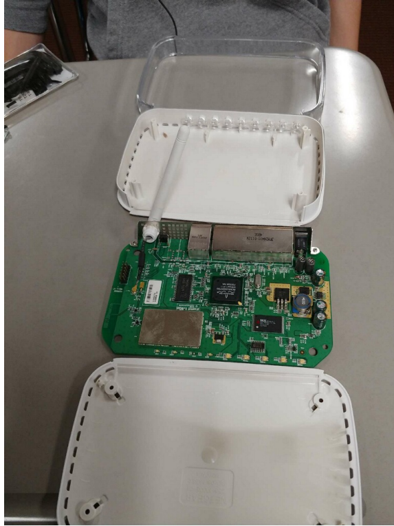
Full disassembly of router
